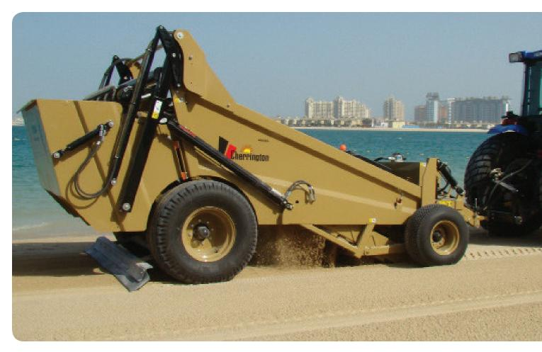
The Cherrington 4600XL is fast, rugged and dependable with only 3 bearings on the conveyor system and no revolving belts, tines, or screens for amazingly low maintenance. A galvanized screen bed and loading paddles, high-speed stainless steel screens, and carbide glide pucks make for a long life and smooth, quiet operation.
