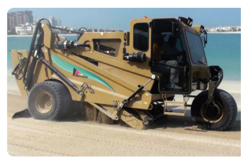
We have combined the proven isolator Lift and Screen Method with state of the art technology and modern, innovative design to bring you the new Model 5500 Beach Cleaner.
