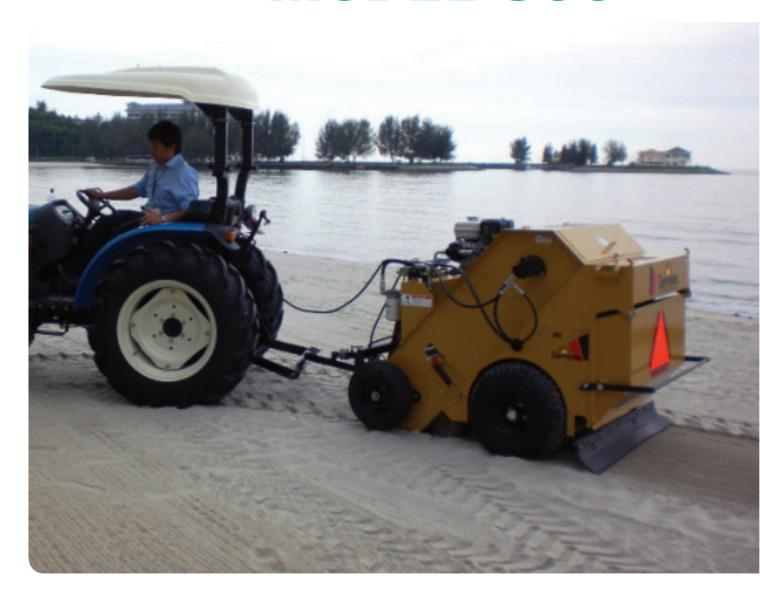
The Model 800 is designed to work with ATV's, utility vehicles, and compact tractors, so it is the perfect choice for anywhere sand cleaning is needed on a smaller scale.
